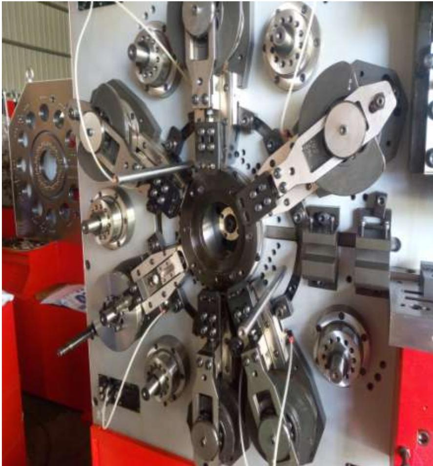
Slides of our machine equipped with dual CAMs, which guarantees long life of inner mechanism.
