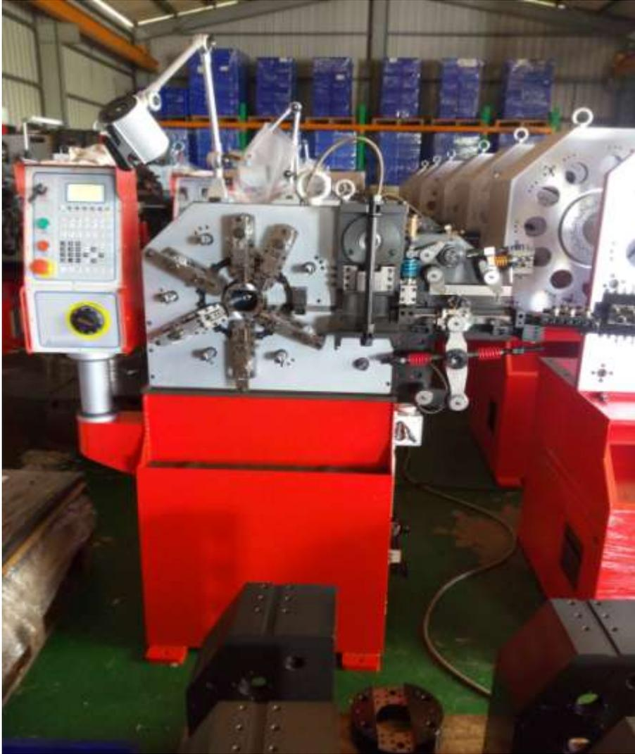
in Amax machines the motor is positioned in the top of machine, so it doesn't require such a large transmission mechanism to send power from motor to the moving mechanisms.
